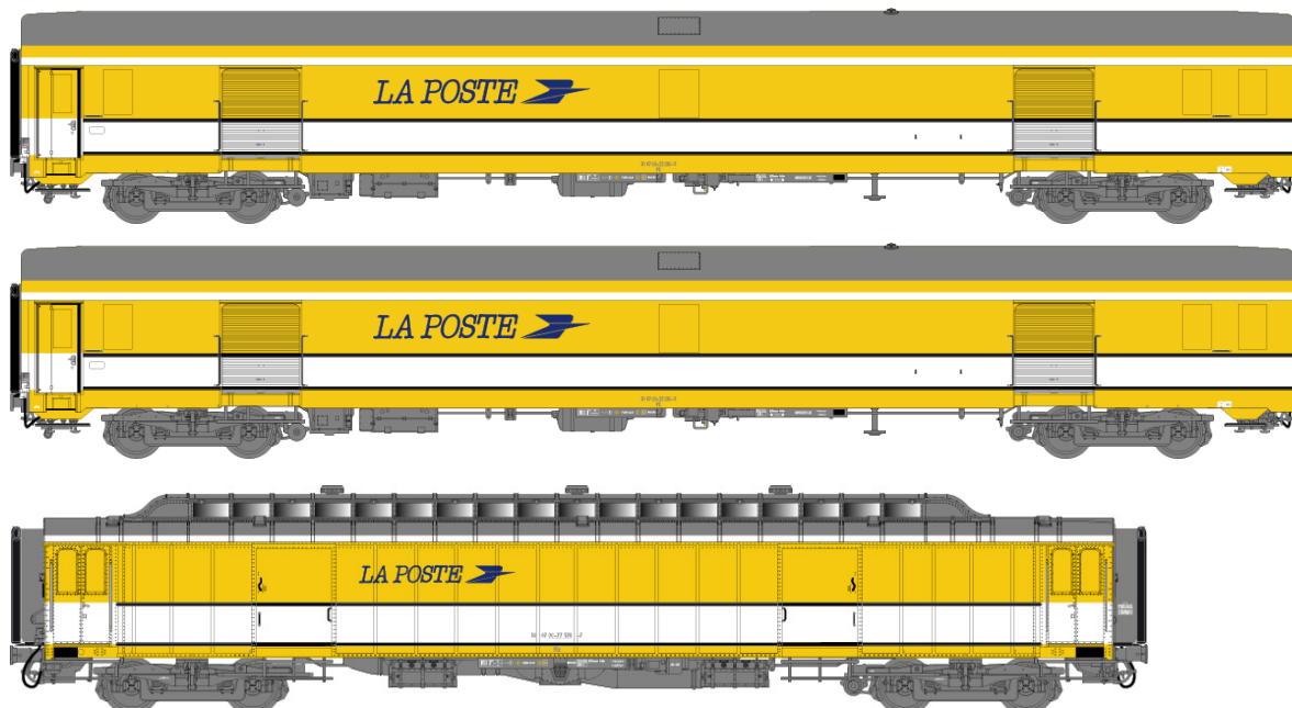
Set 40 425 PA UIC + PA UIC + Pez DCEM caisse jaune/blanc, toit gris, bogies Y24x, intercirculation UIC Ep.V
